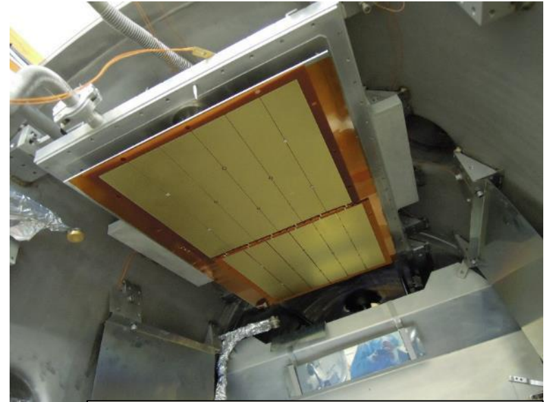
Compass Thick-gem PC coating (CsI)
