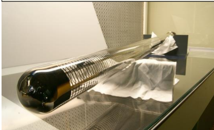
Titanium (conductive) spirals on CLOUD UV sabre
