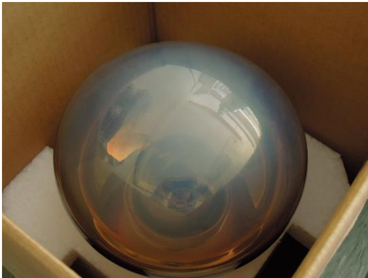
PM wavelength shifter coating (TPB)
