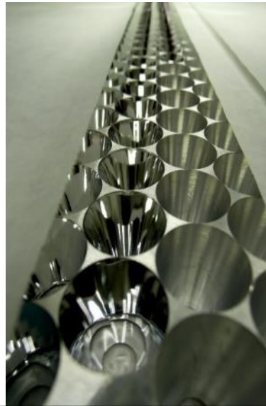
Mylar foil coating for NA62 RICH optical feed trough
