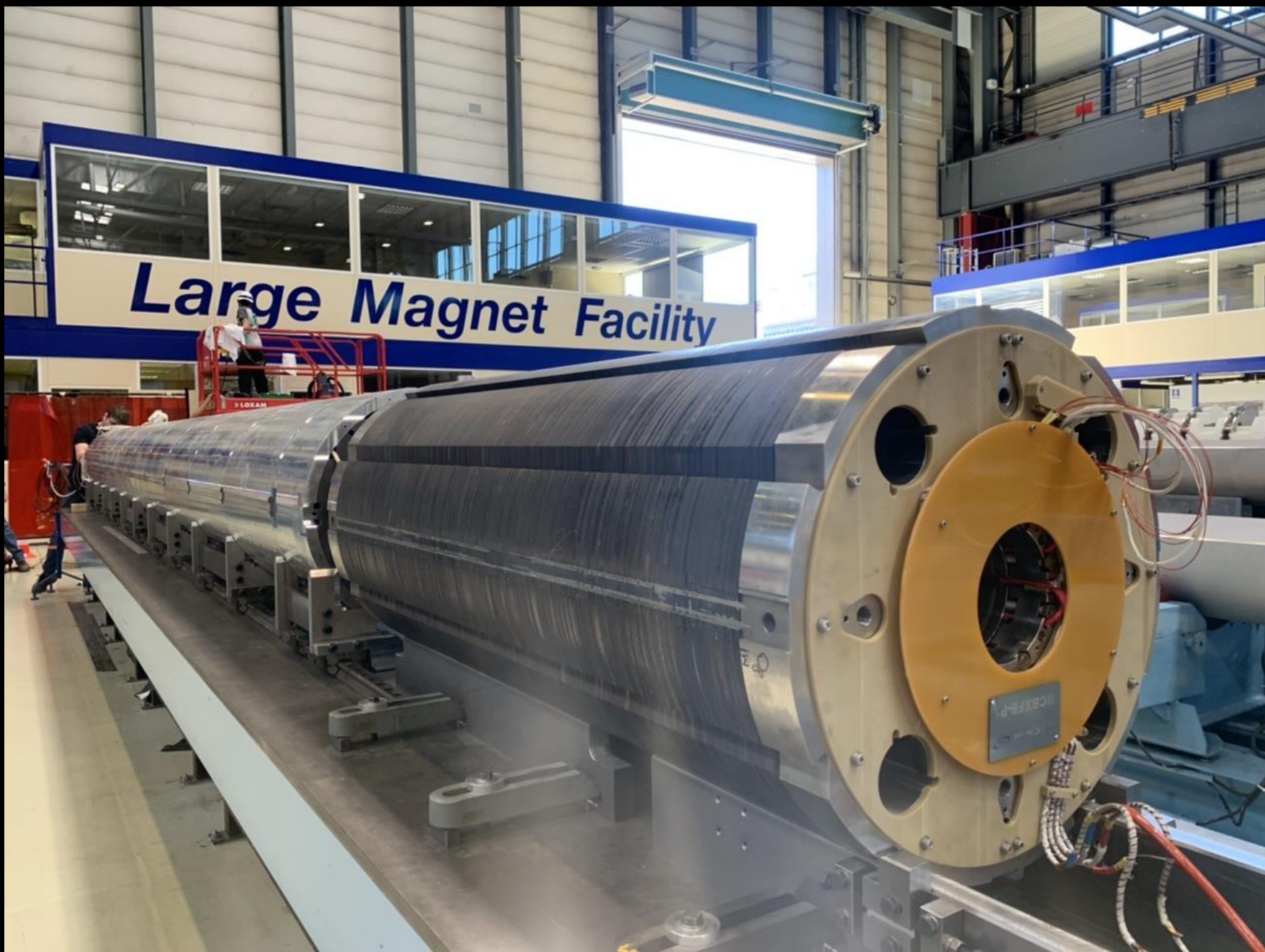
June 2022: MQXFBP2 and corrector MCBXFBP1 on the alignment bench
