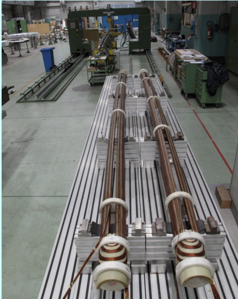
R&D on SC magnets with curved coils
