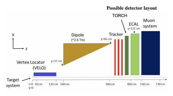
Angular acceptance:  $20 \to 260$  mrad (geometrical efficiency  $\sim 40\%$  for  $\tau \to 3\mu$ )
