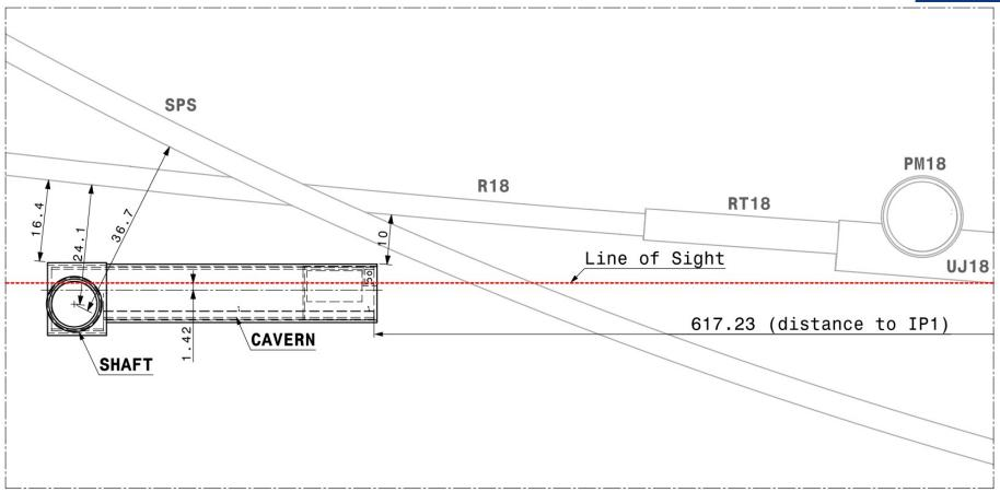
Previous design had a connection from the FPF to LHC (as an emergency escape route). After discussing with HSE this has now been dropped, and replaced with a safety corridor (over pressure), which allows to get from the end of the cavern to the elevator/stairs in a safe way.
