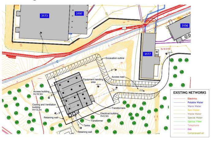
Update in the layout of the access road to avoid interference with existing shallow underground networks
