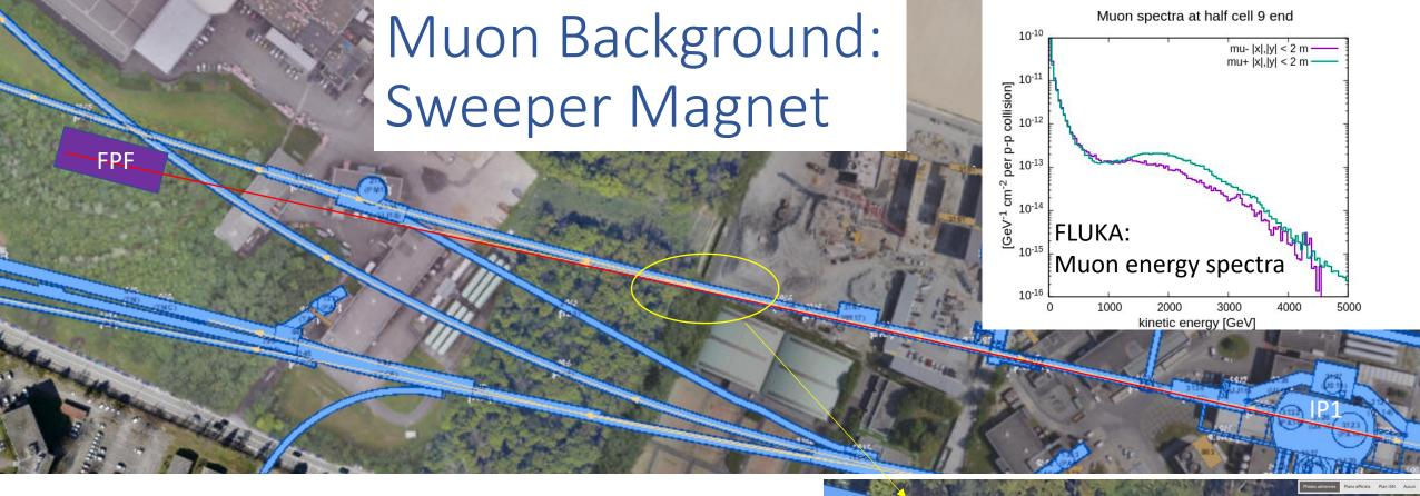
Placing a sweeper magnet on the LOS can deflect these muons and reduce the background.
