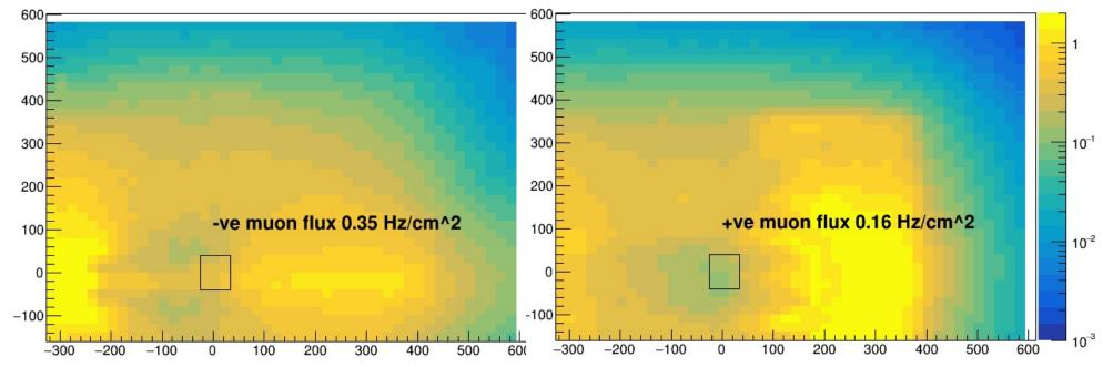
FLUKA muon flux at start of FPF (617m from IP1). Baseline HL-LHC crossing angle of 250urad would push the LOS ~16cm to +ve x in these plots. (LHC tunnel would be at at -1300cm on these plots scale)
