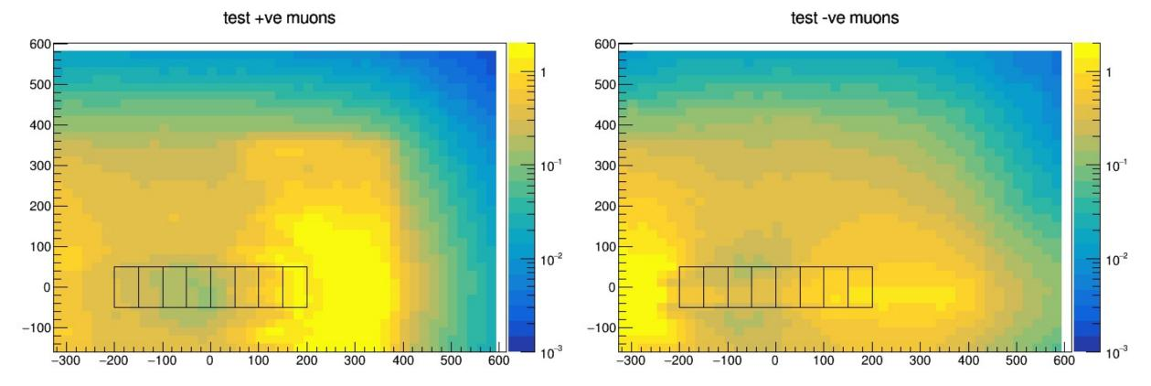
Looking in slices 0.5m wide, 1m high, covering region +/-2m away from the LOS in horizontal plane Muon flux from FLUKA simulation in Hz/cm<sup>2</sup>
