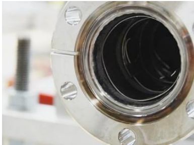
Witness samples placed at the entrance of the pipe
