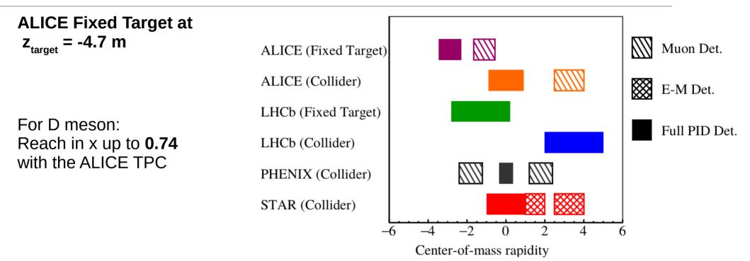
ALICE Central Barrel (CB) in a fixed-target (FT) mode → access to backward rapidity and high negative  $x_F$  domain
