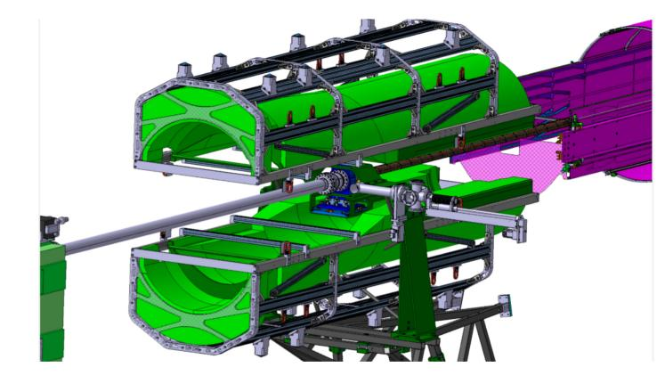
ITS support in open position at  $z \sim -5m$ , to allow for interventions on the ITS during EYETS
