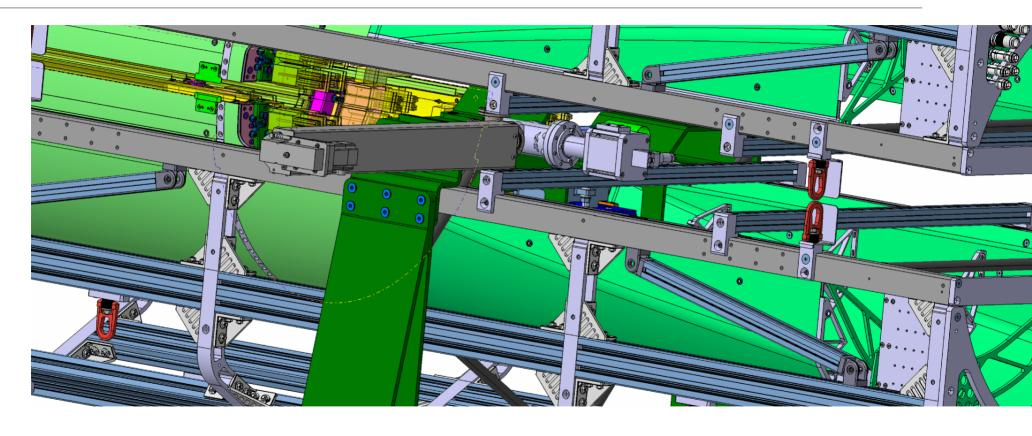
Integration with so-called miniframe (ITS support) seems feasible with target system located in horizontal plane
