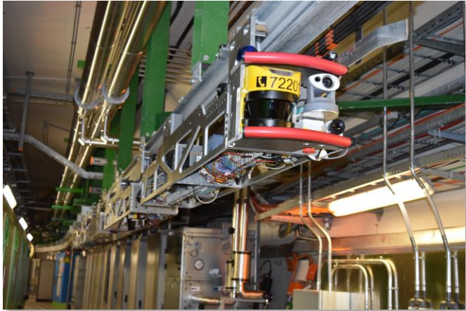
Train Inspection Monorail (CERN made)
