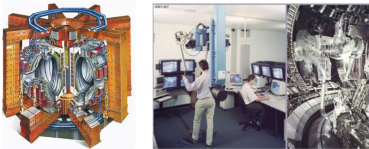
JET Torus (left) and remote handling approach using the MASCOT system
