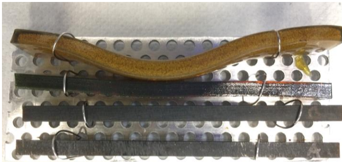
Protective covers for magnets
