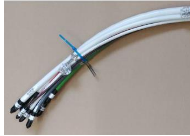
Cables for high-rad areas
