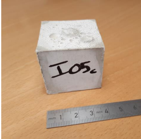
Magnet spacers (grout)
