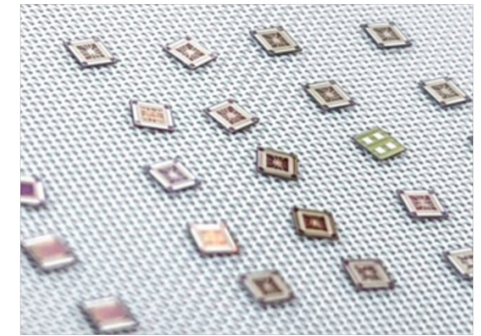
TPSCo 65 nm: test structures
