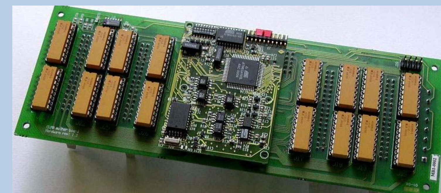
Left : ATLAS sub-detector motherboard with on-board ELMB for front-end electronics configuration, voltages, currents and temperatures monitoring, and local reset of the motherboard Top: ELMB mounted on its dedicated motherboard for general purpose usage
