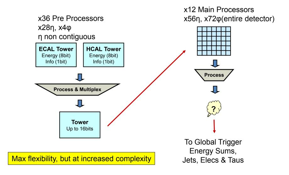
2.4Gb/s input forces processing area to be spit over 2 FPGAs, albeit with large (8-12) tower overlap
