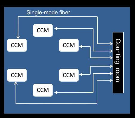
In the existing system a Clock and Control Module (CCM) controls 72 data channels.
