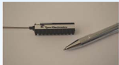
Parallel Optical Engine Tx/Rx (12 channels, 10 Gbps/channel)
