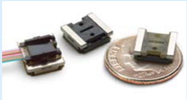
Parallel Optical Engine Tx/Rx (12 channels, 12.5 Gbps/channel)
