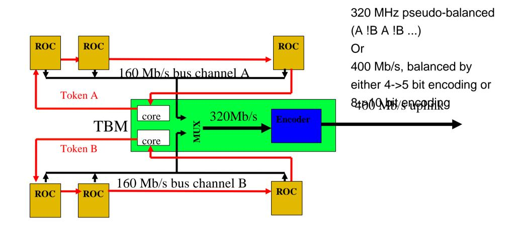
Forward detector has one fiber per two modules: separate MUX
