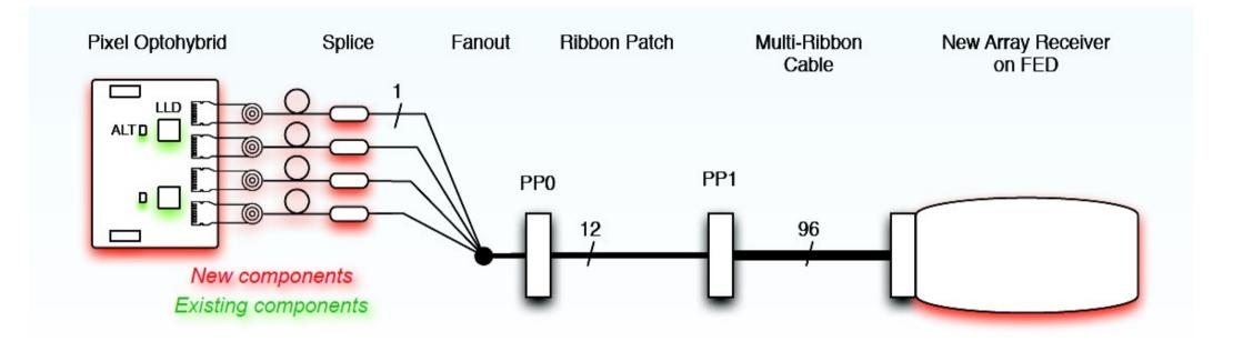
New optical hybrids, existing laser driver and level adapter chips, new lasers
