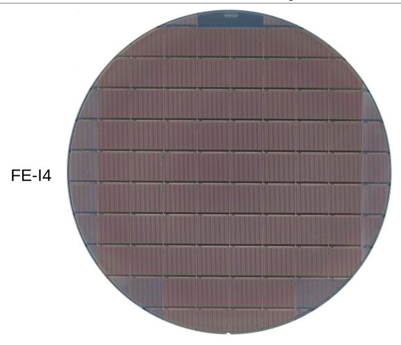
N-on-p pixel sensors on 6" wafers (lower cost pixel sensors for larger detectors)
