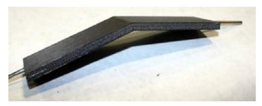
I-beam prototype for inner 2 layers (shared support structure a la Alice)
