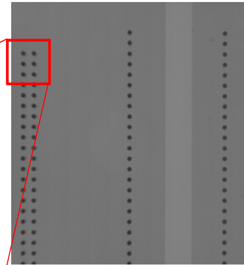
X-ray images 25µm bumped chips (slightly tilted chip left)
