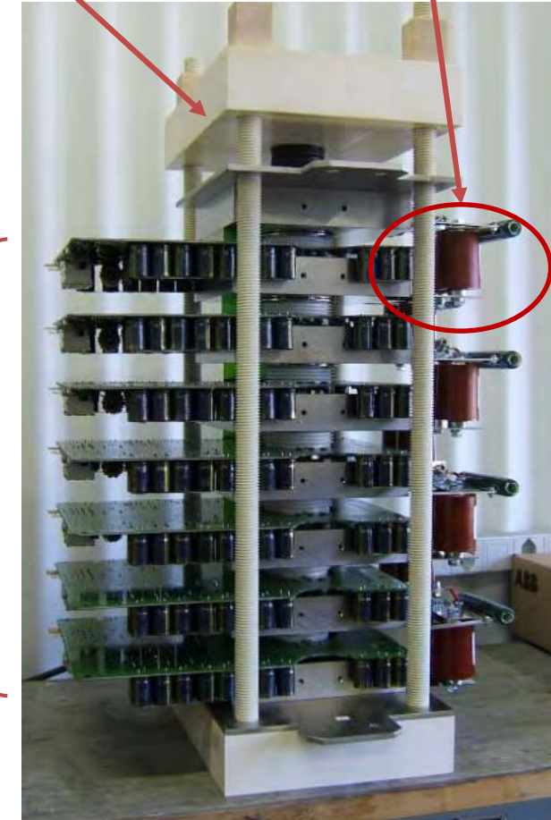
example: ABB switch assembly rated 12 kV/300 A-7x IGCT switch rated 4.5 kV
