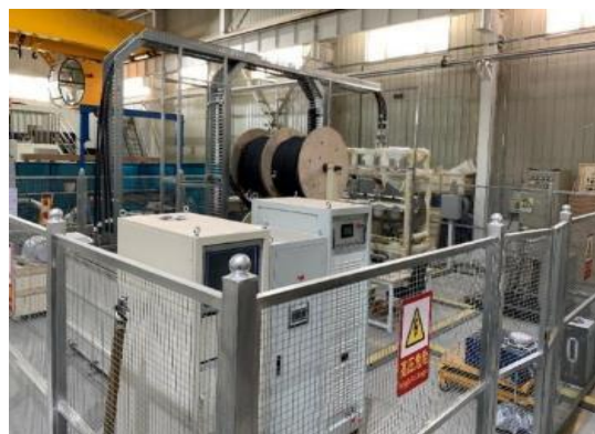
Kicker power supply test with real load
