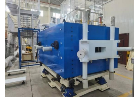
Superferric bending magnet with warm iron
