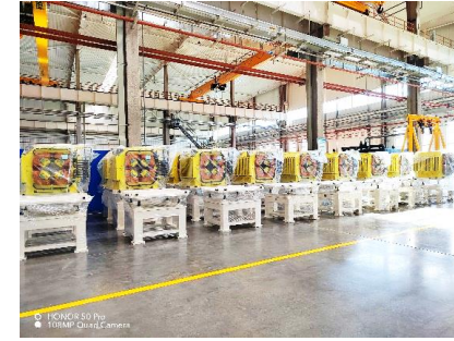
Fast ramping bending and quadrupole magnets of BRing
