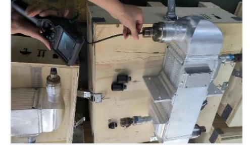
The test of negative pressure heat exchanger
