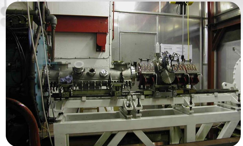
RFQ directly connected by 15.775 cm drift with first Drift tube tank
