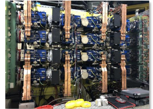
Newly installed H- injection (top) and pre-LS2 multi-turn injection (bottom)
