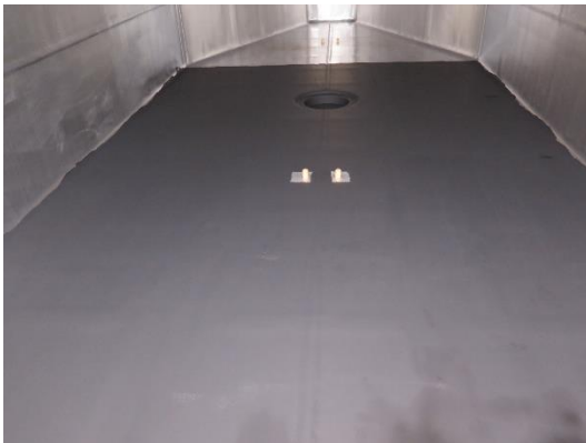
Resonator 4: treated with Aquadag
