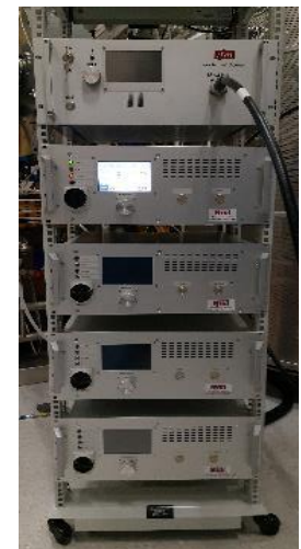
Defect transformer in microwave amplifier No more support New solid state version
