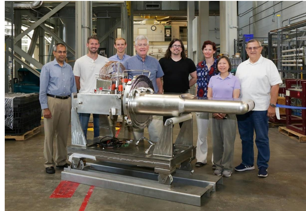
2 MW Target Module (1 st target station)
