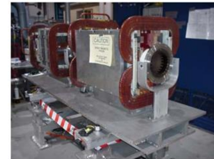
Figure 8: Long Injection dynamic bump magnets with Beam Pipe and Bellow.
