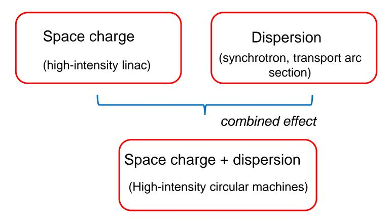
➤ Beam dynamics in high-intensity circular accelerator are subject to **combined effect** of space charge and dispersion
