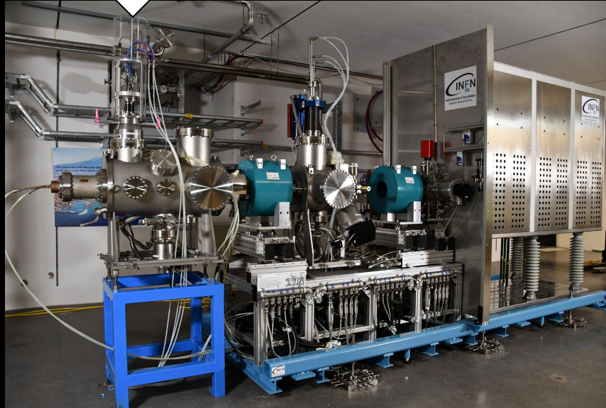
MICROWAVE DISCHARGE ION SOURCE (INFN Catania) [M.ESHRAQI et al., 2020, J. Surf. Investig. 14]
