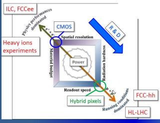
Basic applications are optimized for two different realms of interest : electron and hadron colliders → different optimizations/requirements (pp: radiation hardness, speed; e+e-: granularity, material budget)
