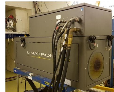
SAPHIR Linatron (X-ray from 6 MeV to 9 MeV)
