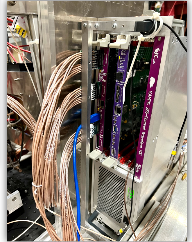
64 channel SAMPIC digitiser, J. Maalmi, D. Breton et al., CAE Saclay
