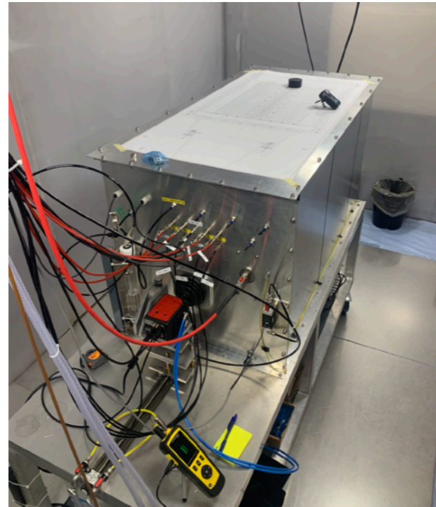
LIME inside the faraday cage
