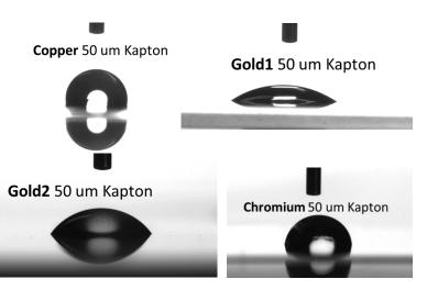
• Surface roughness — In the order of few 100 nm for all the foils except for Chromium which is few nm
