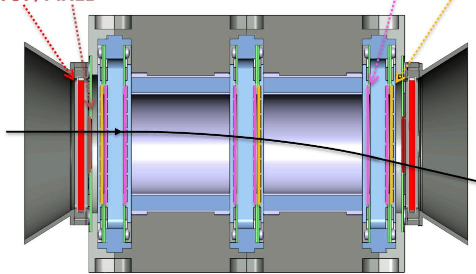
**StripY**: measure the particle direction in Y with an angular resolution ~0.2°
