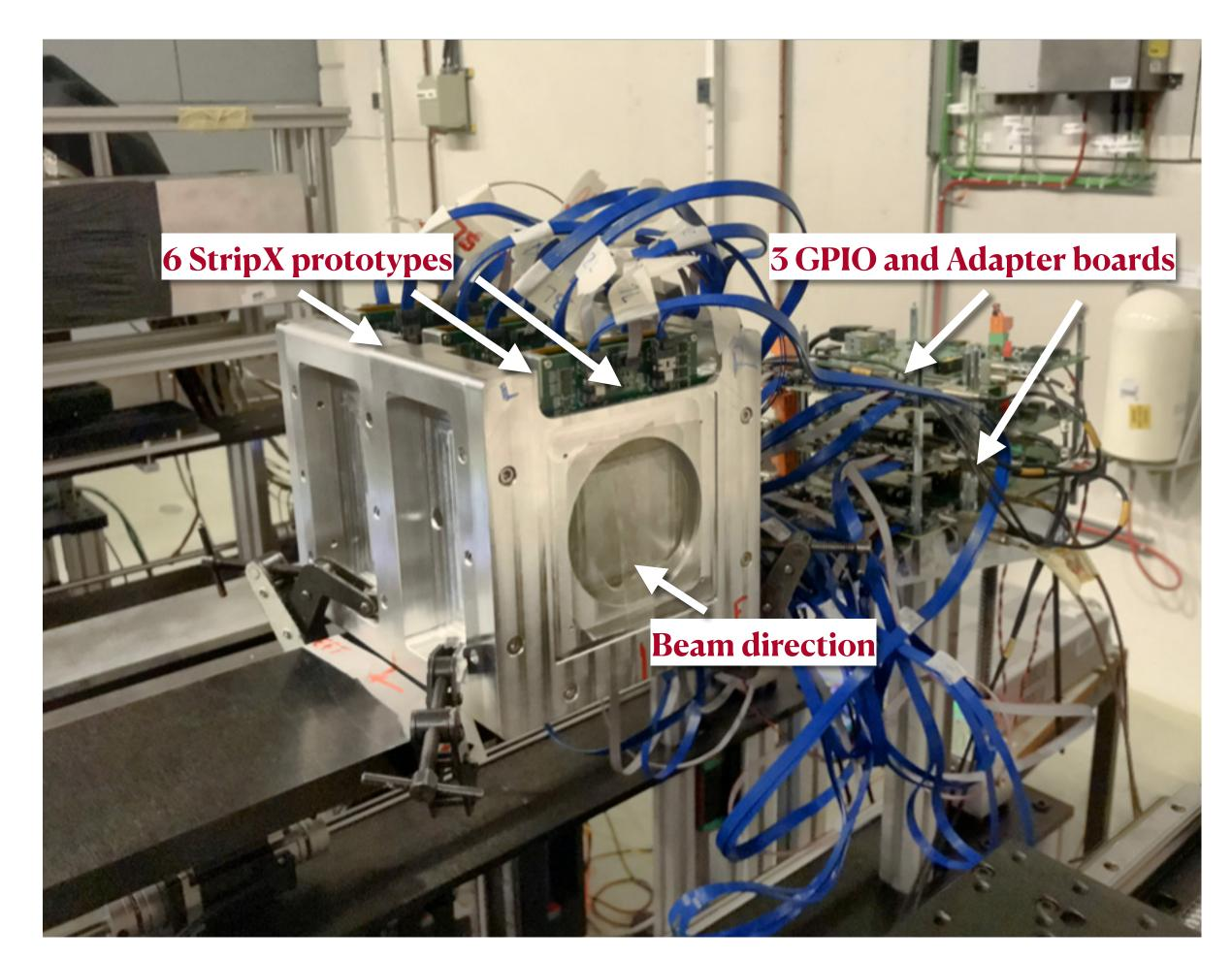
StripX detectors inside the experimental area of T9 beam line.
