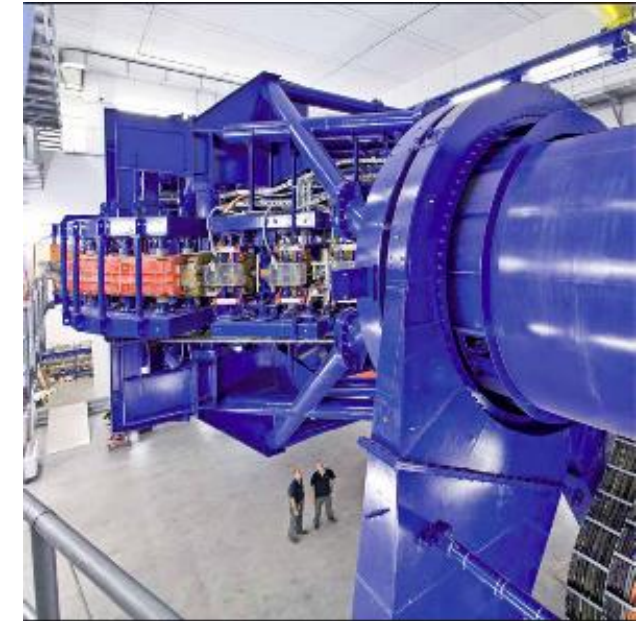
The ion gantry of the Heidelberg Ion Therapy facility: 600 tons
