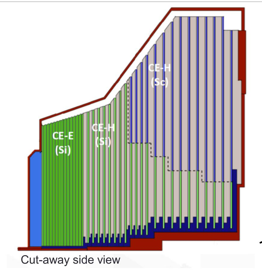
Particle Flow Calorimetry
