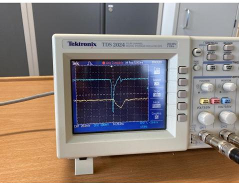
More improvements are being made, including a logical output. This will be used to connect several tanks on 1 microcontroller allowing to measure the time differences with a precision of about 4 ns. A bachelor student is working on a project characterizing these detectors and to develop a directional reconstruction including uncertainties
