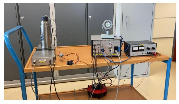
3D printing makes life a lot easier. We now print a replacement for the cap and in principle the inside can be adjusted for different photosensors. The PM is not directly in the water but there is a small glass between water and PM which enables all of this. Lots of new experiments are possible. In addition: Contrary to the scintillator-plate this is a 3-D detector thus suddenly inclined incoming muons can be seen as well.
