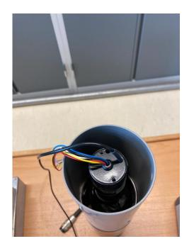
Our original version consisted of a modification of the lid so that the PMT could see the water, through a piece of glass. All properly sealed and light-tight. Standard PVC tubing to protect the PMT. Rather labor intensive to make...
