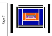
**magnet** bends the trajectories of particles so can can estimate their momentum; **electromagnetic calorimeter** picks up electr and photons; the **hadronic calorimeter** measu activity from particles made of quarks a gluons; and the **muon spectrometer** tells where muons passed.
