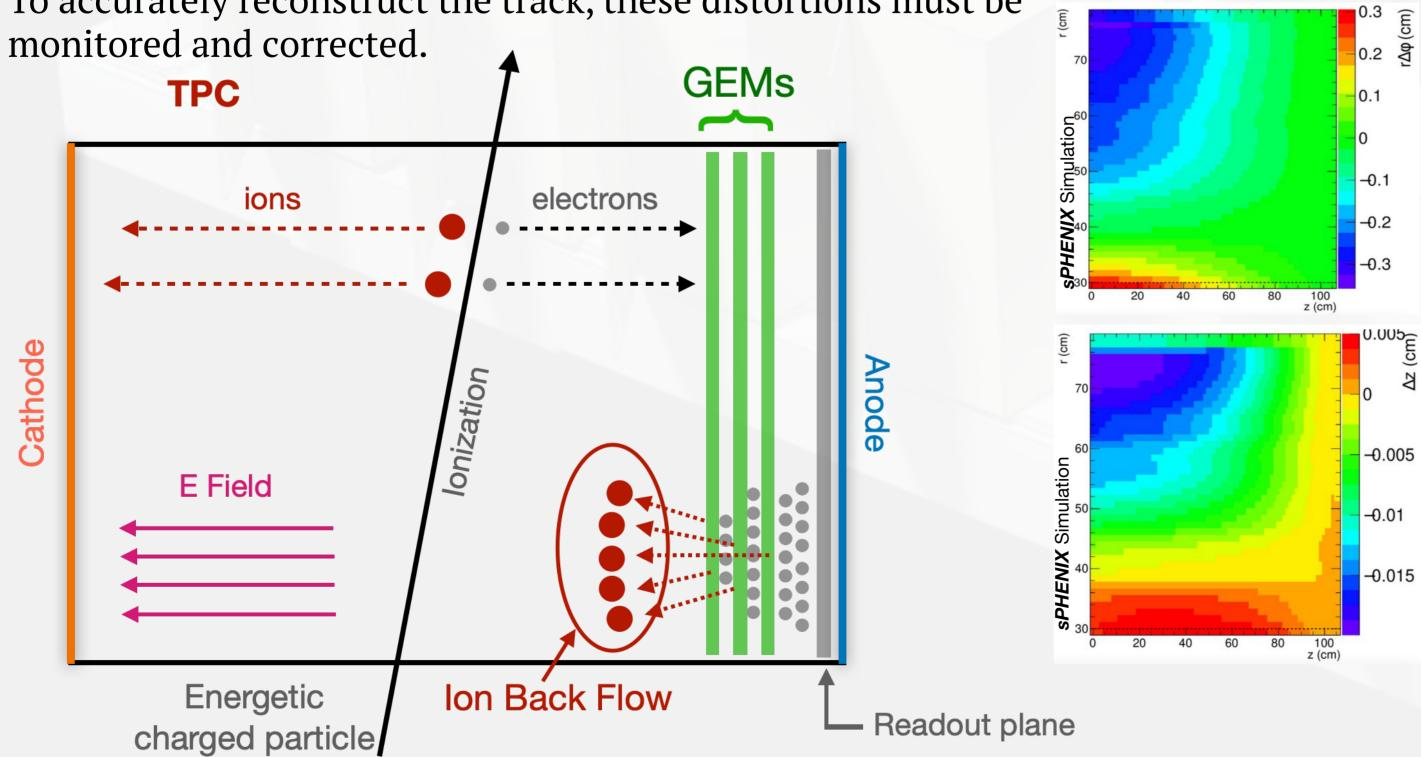
Need to correct for the distortions in the TPC for precise track reconstruction
