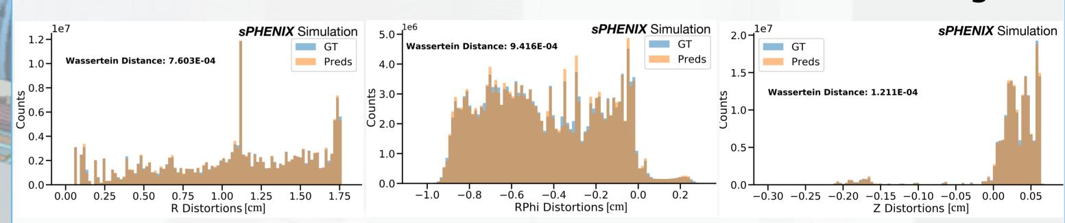
Simulated distortions in the TPC (cm) shown in blue for brute-force calculations on simulated space charge distributions (labelled GT) and in orange for ML-based predictions trained on those simulations (labelled preds) in r, rphi and z axes
