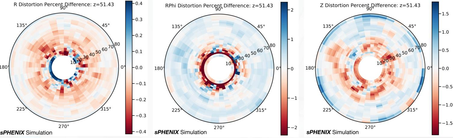
Difference in the TPC distortions (%) between calculated values in simulations and MLbased predictions in r, rphi and z axes shown for a specific value of z (=51.43 cm)
