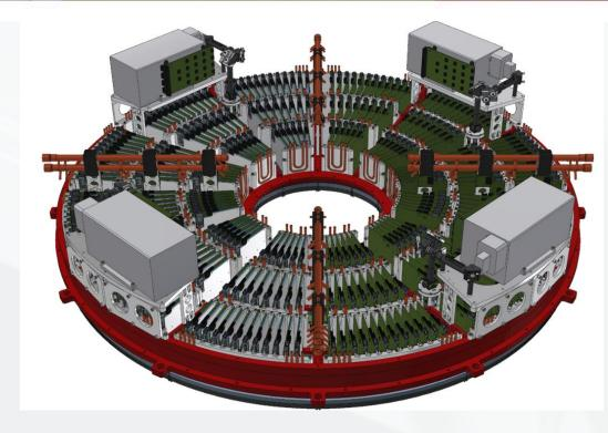
The lasers are mounted at the wagon wheel of the TPC – 4 on each side. Laser light is produced in the optical bench (shown on the right), sent through the two-stage steering, and then enters the TPC gas volume.
