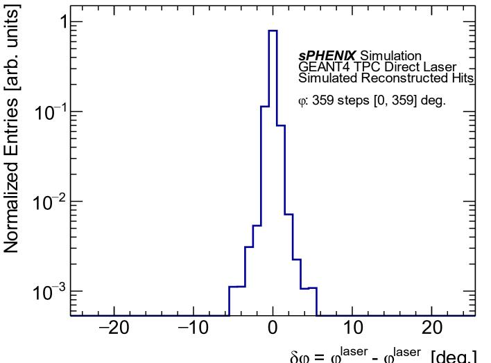
The maximum of the Hough transform method reconstructs 90 % of angles within < 1° error without noise/distortion.
