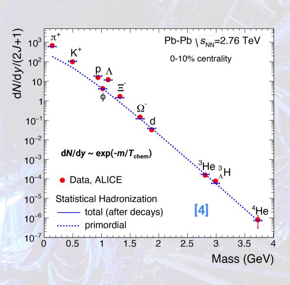
Hadrons emitted from the interaction region in thermal equilibrium when the fireball reaches the freeze-out  $\rightarrow$ Abundances are fixed at chemical freeze-out ( $T_{\text{chem}}$ )
