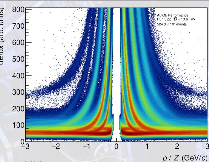
TPC response for pp  $\sqrt{s}$  = 13.6 TeV collisions. The <sup>3</sup>He signal is fitted with ALEPH Bethe-Bloch functions (in black).
