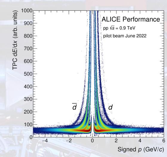
In TPC, PID is performed measuring the energy loss (dE/dx) of particles in the gas as a function of the rigidity. Antideuteron candidates are preselected requiring a dE/dx compatible within 5σ with the expected signal for  $\bar{d}$ .
