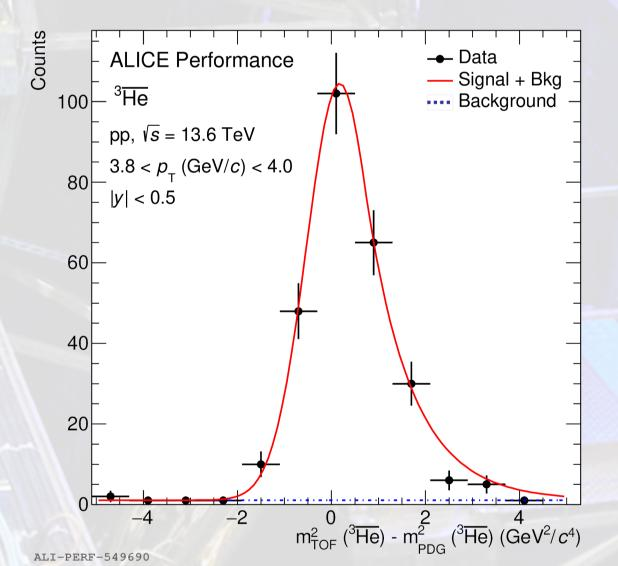
The (anti)helium signal is extracted for different ranges of  $p_T$  (from 1 GeV/c up to 6 GeV/c) in via the TOF detector. The difference between the squared masses is fitted with a function defined as the sum of an asymmetric gaussian function (in red) for the (anti)helium signal, and a constant function (in blue for the background).
