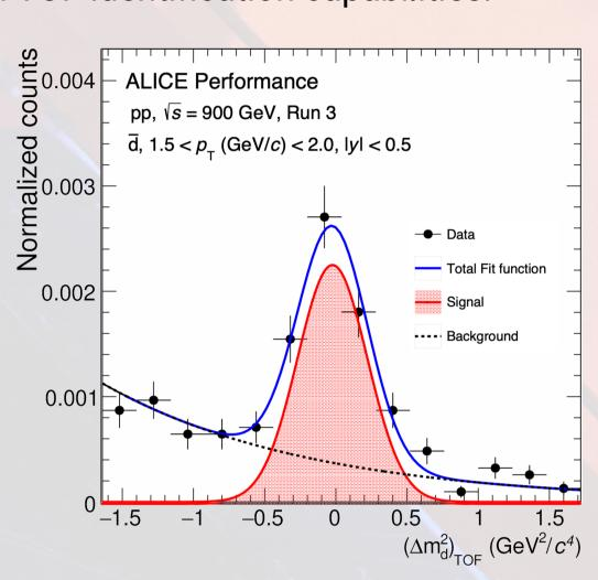
The antideuteron yield is extracted by fitting the distribution of the difference between the squares of the mass reconstructed using the TOF information and the nominal mass.
