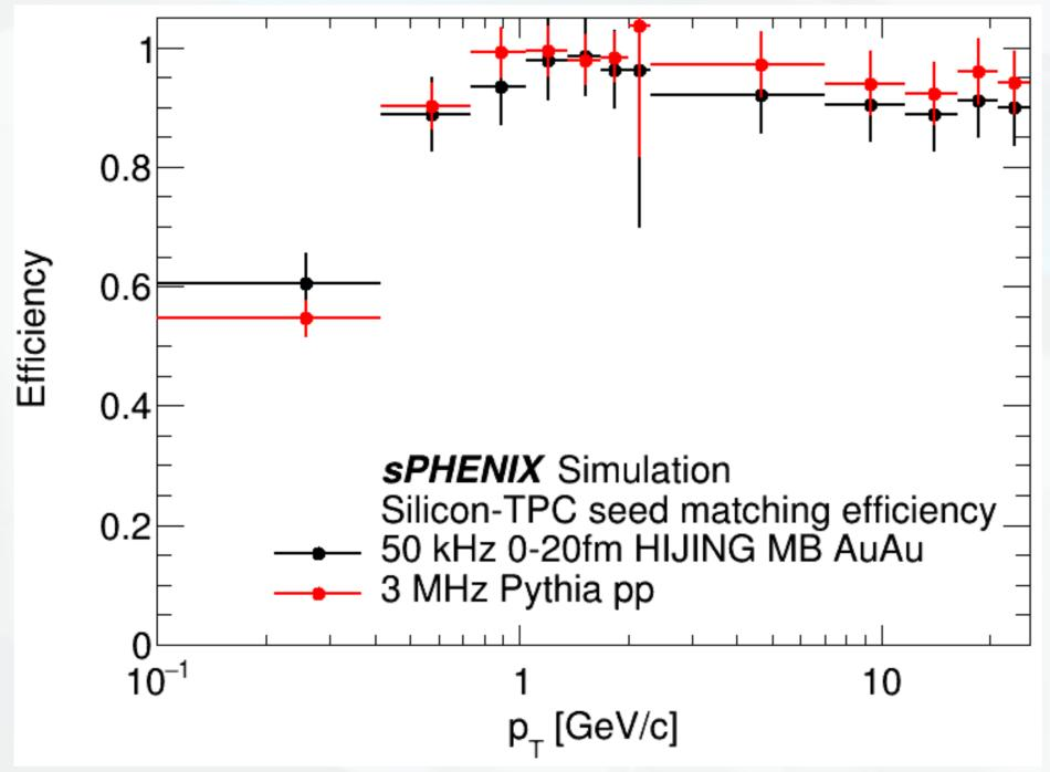
If no silicon seed is found for a TPC seed, a track object is made anyway, containing only the TPC seed. This is useful for K<sub>s</sub> and conversions, both of which may not produce any hits in the silicon detectors.
