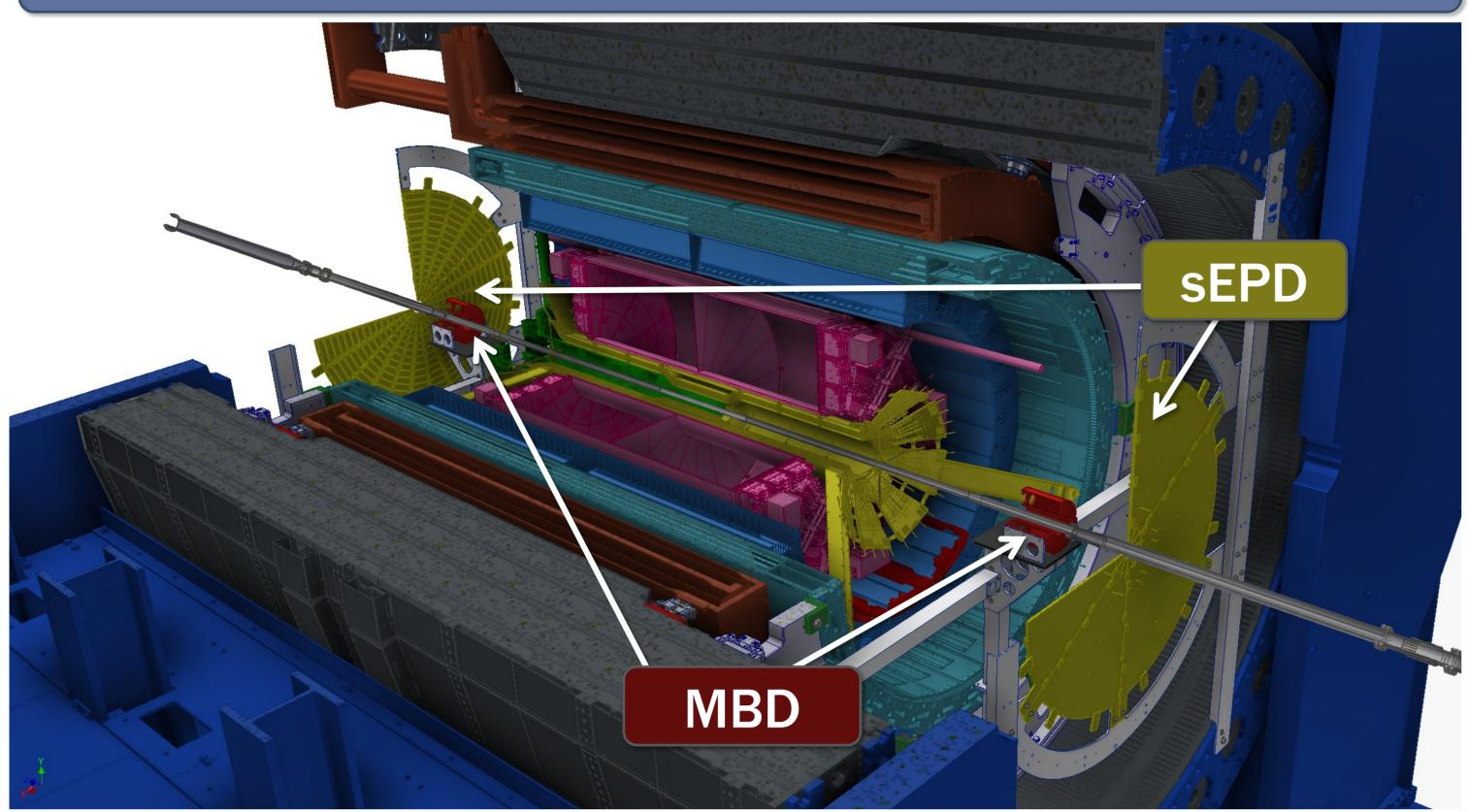
The subsystems used for the  $\psi_2$  determination are the Minimum Bias Detector (MBD), and the sPHENIX Event Plane Detector (sEPD), covering  $3.5 < |\eta| < 4.5$  and  $2.0 < |\eta| < 4.9$  respectively. The MBD  $\psi_2$  results are with Au+Au at 200 GeV data, while the sEPD  $\psi_2$  is with HIJING and flow after burner.
