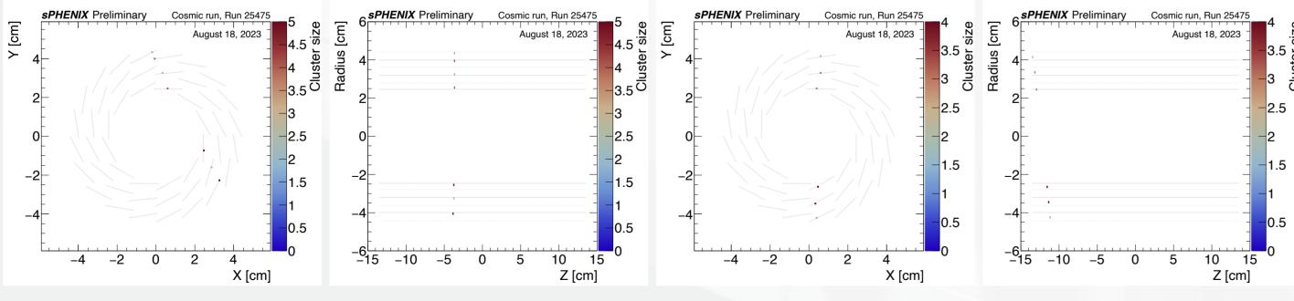
■ Shown in the figure to the right is a cosmic candidate passing through all tracking sub-detectors: the MVTX, the intermediate tracker (INTT), the time projection chamber (TPC), and the time projection chamber outer tracker (TPOT). This confirmed the readiness of the MVTX readout system and the external synchronization with other sub-detectors
