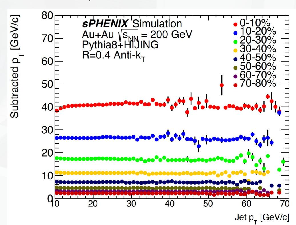
The total energy of the UE subtracted from the jet is plotted vs the subtracted energy of the jet for each centrality bin as a different color.
