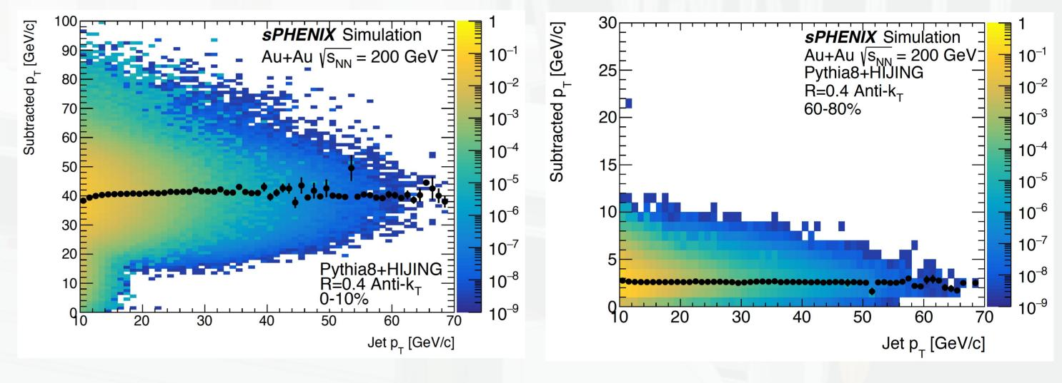
The total energy of the UE subtracted from the jet is plotted vs the subtracted energy of the jet for central events (left) and peripheral events (right).
