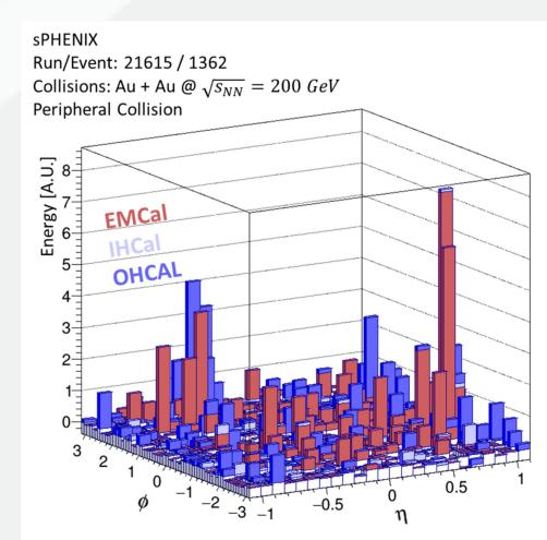
First look at jet reconstruction with data from calorimeters in run 2023.
