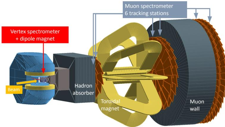
**Figure 1.** View of the NA6+ experimental apparatus. The beam is coming from the left side.
