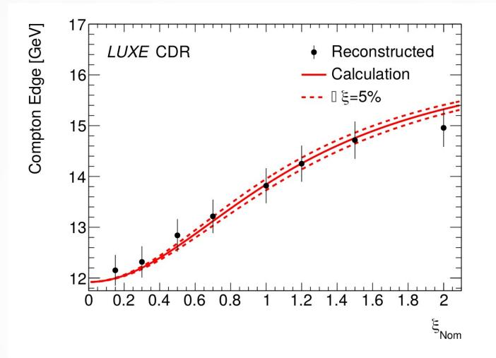
Compton electron edge upper kink position from simulated analysis as a function of the nominal  $\xi$  value. The red solid line shows the theoretical prediction. The dashed lines show the impact of a 5% uncertainty on the laser intensity. The black circles show the anticipated data result based on the analysis. The uncertainty shown is dominated by an energy scale uncertainty of 2.5%, a statistical uncertainty corresponding to 1 h of data taking is also included but negligible.
