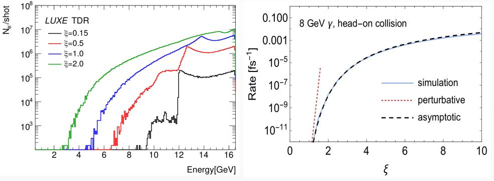
Simulated expected rates for each of the two interactions. Left shows the energy spectra of electrons after radiating through non-linear Compton scattering. Right shows the changing rate of multiphoton Breit-Wheeler, beside an extrapolation for the perturbative solution at low  $\xi$ .
