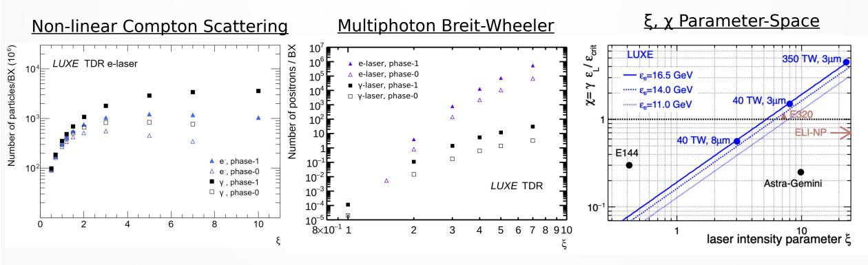
Left: the numbers of electrons scattered and photons radiated per bunch crossing in the e-laser mode of LUXE for changing ξ parameter. Center: The numbers of positrons (and electrons in a pair) created per bunch crossing in the e-laser and γ-laser modes, for changing ξ parameter. Beam energy assumed at 16.5 GeV. Right: the parameter space in ξ, χ, spanned by LUXE
