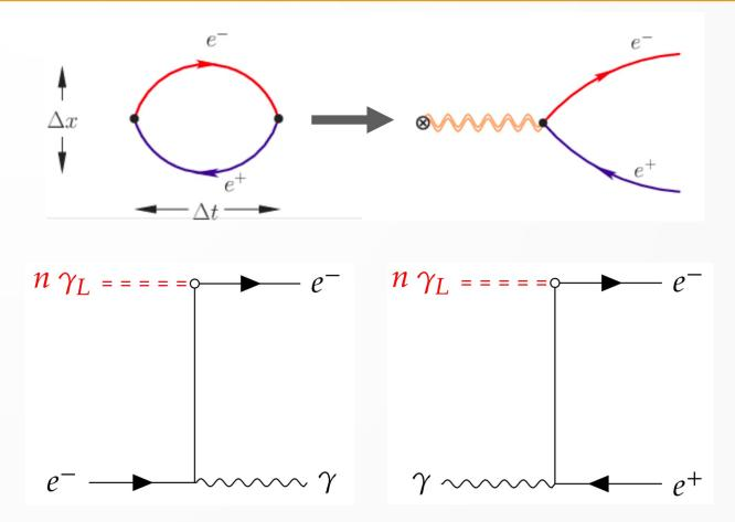
The two interactions of interest: Non-Linear Compton Scattering (left), Multiphoton Breit-Wheeler Process (right). The two can occur immediately after one another, in a 'trident' process
