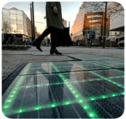
each there's Inside tile an electromechanical which system, transforms vertical the small movement produced by people walking into a rotating movement that drives a generator.
