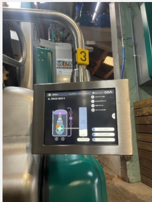
Figure 16 Machine monitor showing how this cow has one breast that is not producing good milk.
