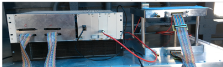
Detectors assembled with readout and high voltage electronics system
