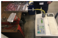
Detectors assembled with readout and high voltage electronics system
