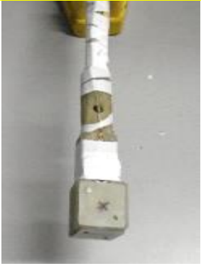
3 SQUIDS mounted on FRP in 3 orthogonal directions
