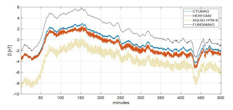
Correlation of the temperature variations and magnetometer output oscillation is visible in time domain as well as in frequency domain, close to 5 mHz.
