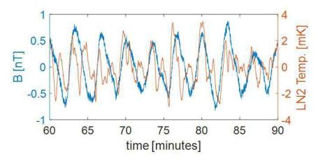
PT1000 (non-cryo) At 77 K : 6 mKpp  $\rightarrow$  2 nTpp peaks @ 5 mHz
